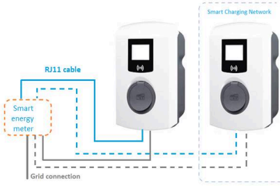
Figure 5.2: Active Load Balancing with energy meter (P1 port)
