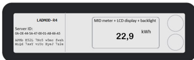
Figure 3: The Eichrecht compliant energy meter display with kWh value and public key
